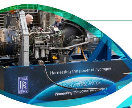
Rolls-Royce and easyJet achieved the world's first run of a modern aircraft engine on hydrogen proving the fuel can be combusted at conditions that represent maximum take-off thrust.
