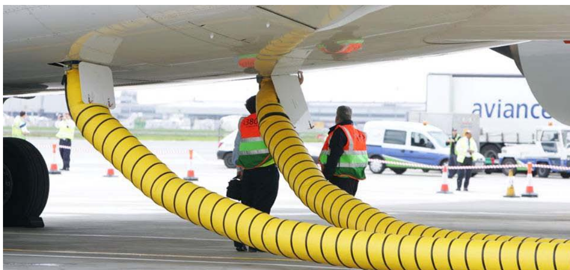
Figure: Example of Preconditioned Air
