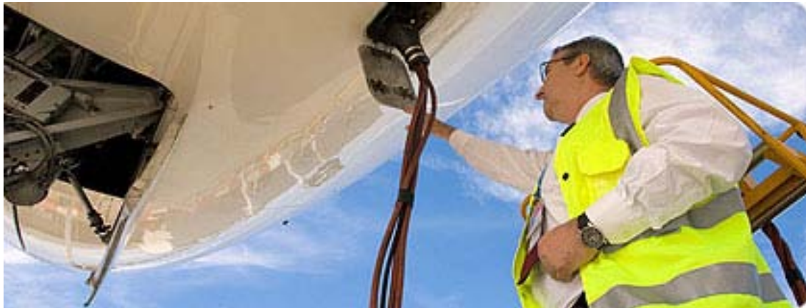
Figure: Example use of FEGP at Stansted airport
